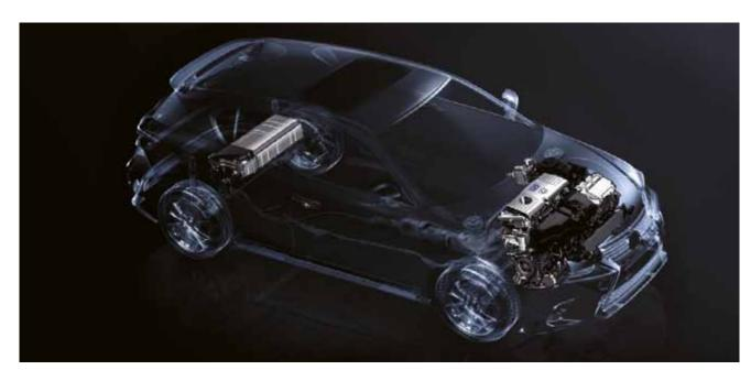
For astonishingly smooth performance and low  $CO_2$  emissions, the CT 200h orchestrates a combination of super-efficient 1.8-litre engine, high-output electric motor, powerful compact battery, seamless hybrid transmission and power control unit.
